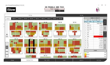
It helps a planner to allocate all container types on board a container vessel efficiently and accurately.
