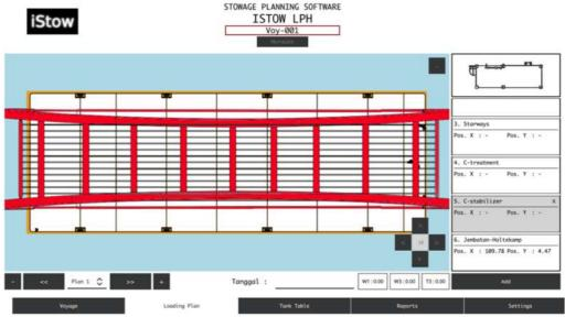
It assists a load planner to plan the loadout of large and heavy objects such as offshore platform, a harbour crane or a bridge, efficiently and accurately.
