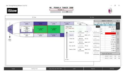
It helps a planner to allocate all types of liquid cargo on board a tanker efficiently and accurately.
